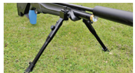
The XM1 with the individual bipod legs fitted to the Picatinny rails either side of the forend
