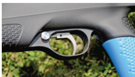
A push-button safety sits in front of the 2-stage trigger, note the bright blue grip
